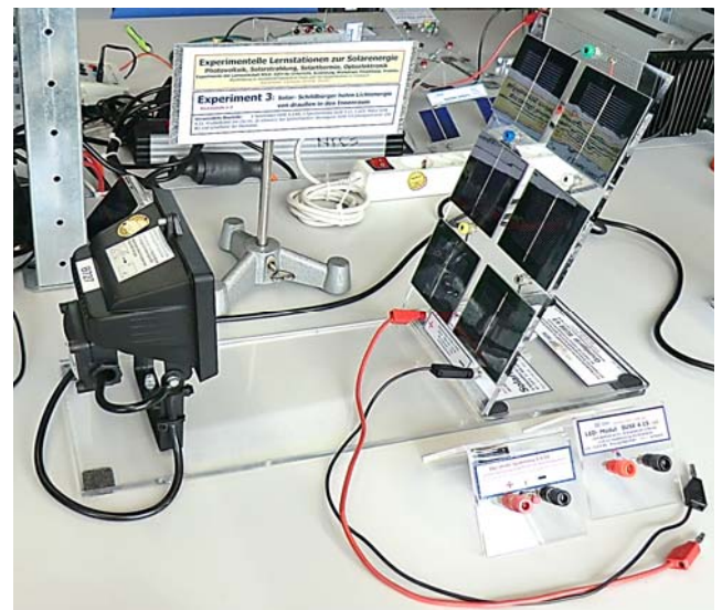
Setting of the experiment A3: On the base plate SUSE 4.0 the solar module SUSE 4.3RB is located, in front of it there are the storage module SUSE 4.12 and the LED module SUSE 4.15
