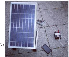
Charging a smartphone with solar module SUSE 4.42 (20 W) and charge regulator SUSE 4.17
