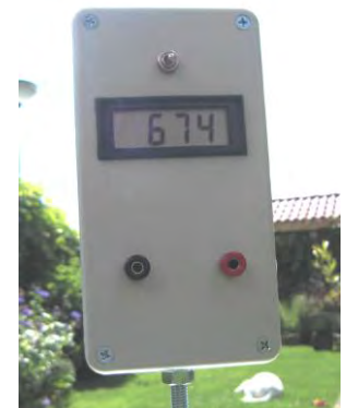
Display of the solar irradiance S = 674 W/m 2 on a slightly cloudy day
