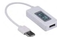
USB measurement technology to measure voltage, current, charge
