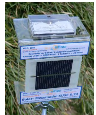
Display of the solar irradiance S = 674 W/m 2 on a slightly cloudy day
