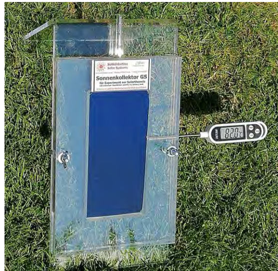
Collector outdoors on a meadow, the thermometer displays the absorber temperature of 82°C.
