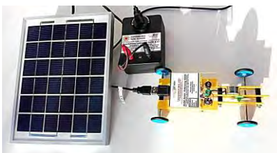
Top: Solar vehicle SUSE SF6USB with solar filling station SUSE 4.51 and DC-DC converter SUSE 4.17
