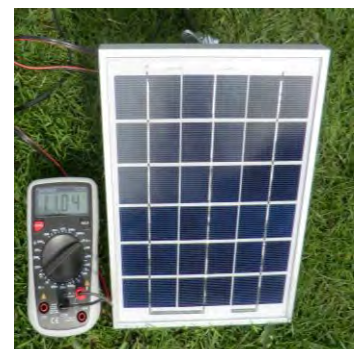
Displayed is the open circuit voltage 11,04 V
