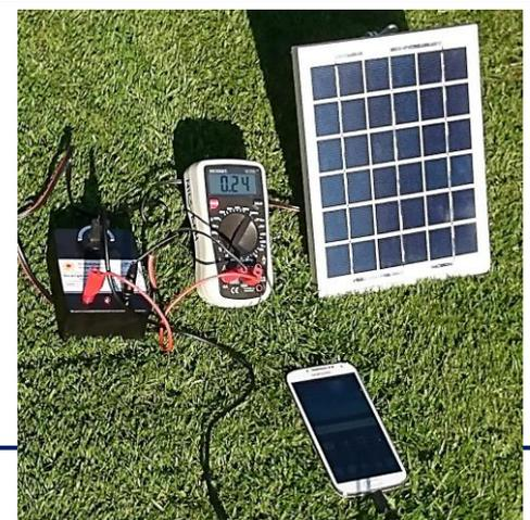
charging module SUSE 4.17. The amperemeter shows the charging current of 0.24 A.
