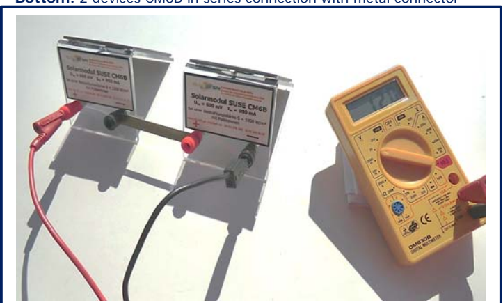
Top: The solar module SUSE CM6B, on the left the solar cell SUSEmod2 Bottom: 2 devices CM6B in series connection with metal connector
