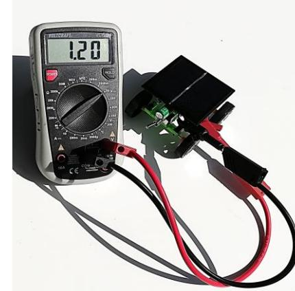
With a voltmeter, the module voltage, the short-circuit current, as well as the charging and discharging of the capacitor can be measured at the vehicle and measurement curves can be created. Here the measurement value of 1,20 V is shown during charging.
