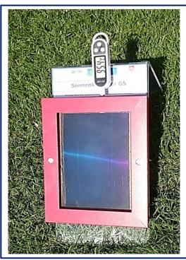
The probe thermometer in operation on a solar thermal collector ES, currently it shows 95.4°C. The measuring tip fits inside the inserting pipe of the collector and is slid under the absorber.
