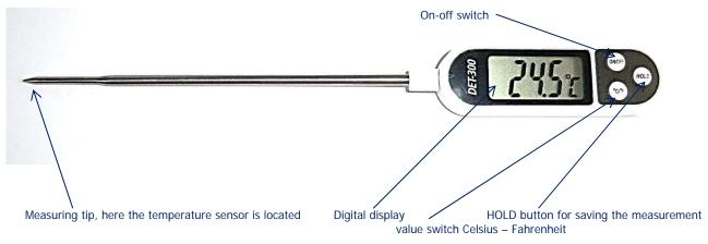
To take a measurement the device is switched on, then directed to the temperature measurement point with the tip, or inserted into the measurement points on the collector respectively. To note the measurement value in a table at the workspace, the HOLD button is pressed, so that the temperature doesn't decrease by the removal from the measurement point.
