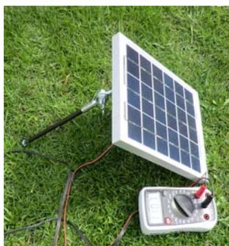
**Top:** Solar module SUSE 4.51, the multimeter shows the open circuit voltage 11.04 V.
