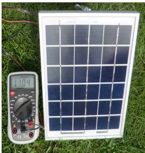
The **solar module SUSE 4.51** is a professional and very robust solar module with 18 solar cells in intern series connection behind glass, framed with a stable aluminum frame. On the module's back side an adjustable positioner is mounted, with which the module can be adjusted continuously in an ideal angle towards the position of the sun on the ground or on a table.
