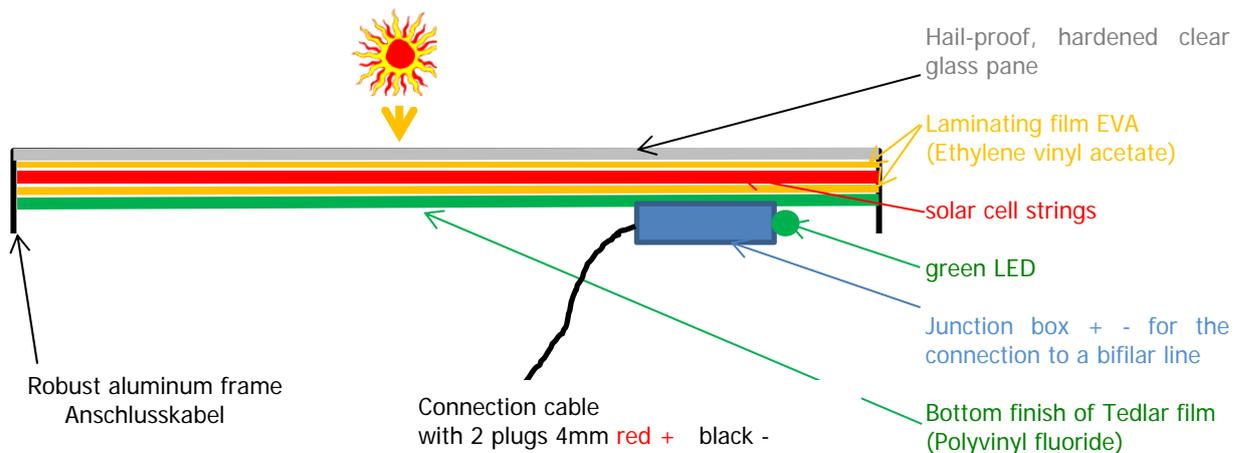
Soldered in the junction box of the solar module SUSE 4.51 is a 1.5 m long bifilar connection cable with two 4 mm bunch plugs **red (positive)** and black (negative), **a green LED** shows operational readiness.
