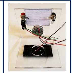
Assembly of jacks, soldering eyelets, switch
